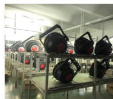
ROKEE LED High Mast Light FL-07-G9 aging (110)
